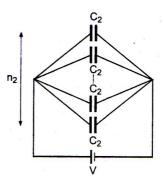
Total capacitance of the parallel combination of capacitors is,
