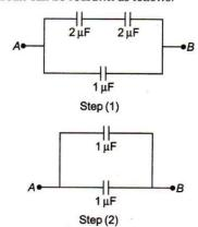
So, equivalent capacitance between A and B  $C_{AB} = 1 + 1 = 2\,\mu F \label{eq:CAB}$
