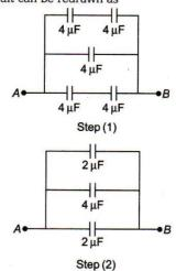
So, equivalent capacitance between A and B,  $C_{AB} = 2 + 4 + 2 = 8 \, \mu \text{F}$
